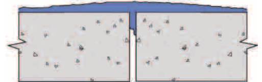
Aqualastic™ bridges cracks to accommodate expansion and contraction from freeze-thaw cycles unlike conventional caulk/joint fill products.
